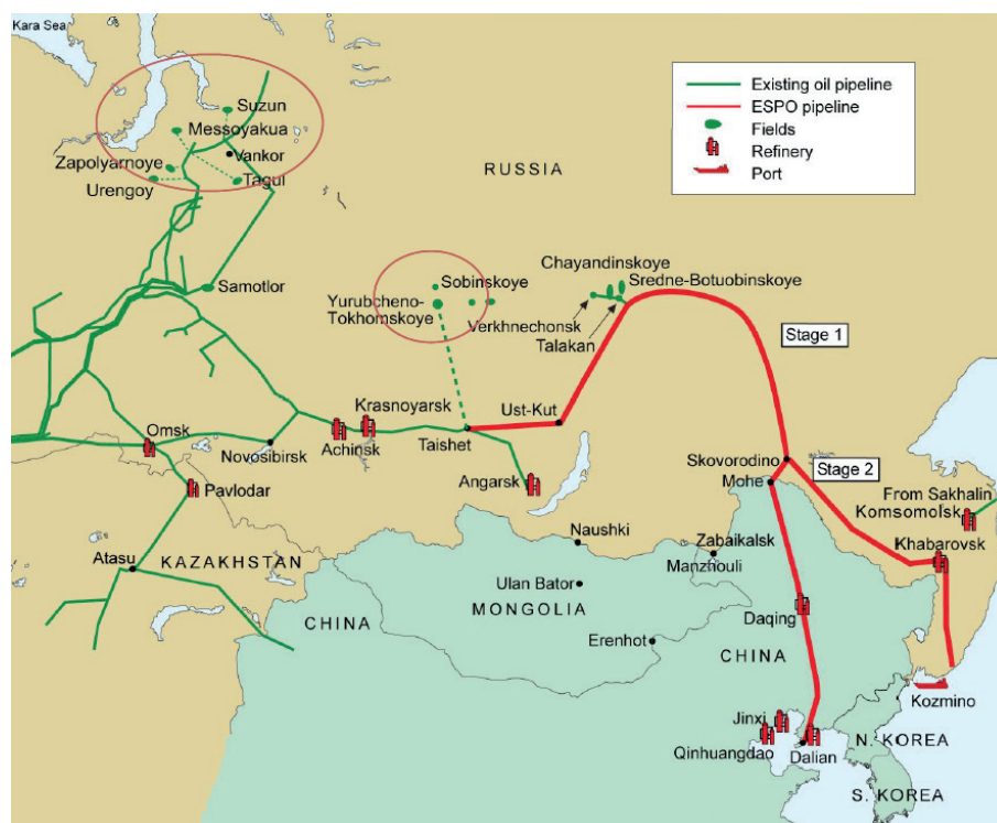
FIGURE 3: OIL FIELDS IN EASTERN RUSSIA AND ESPO PIPELINE (SOURCE: ARGUS)
